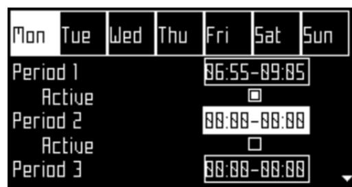
7. Use the numeric keyboard to enter the start and end time values where the cursor is flashing then press .
