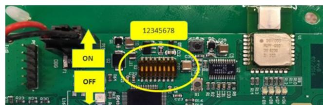
Figure 39: Charging station type switches
