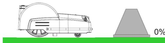
Figure 69: Longitudinal slope of the charging station
