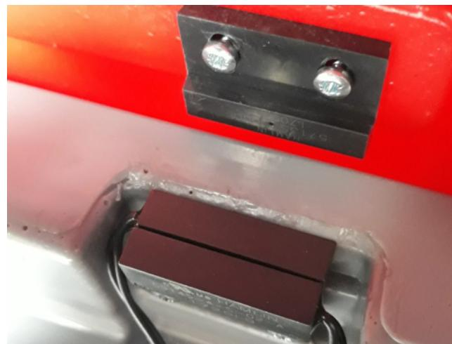
Figure 111: Positioning of magnets and the reed relays
