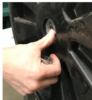
**20.** Tighten up the wheel screw to 65Nm.
