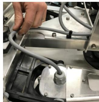
2. Repair any minor damage to the sheathing with tape.
