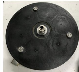
9. Add some glue to hold the washer on the threaded axle.
