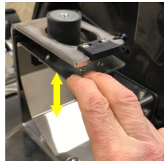
3. Check the movement of the bracket to ensure the correct reverse detection.
