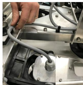
2. Repair any damage to the sheathing with tape.
