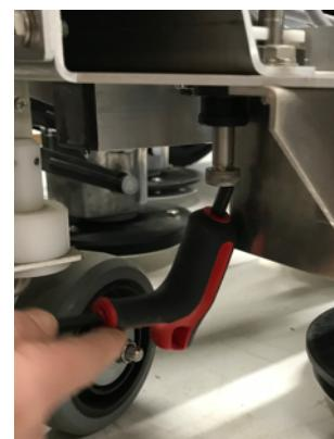
2. Place the new silentbloc in place in the position as shown below.
