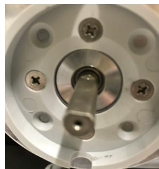
13. Tighten the screw onto the axle using 6Nm.
