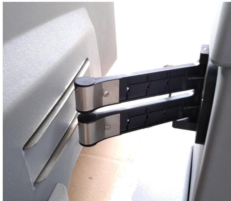
Figure 35: Correct positioning of the charging station and the robot
