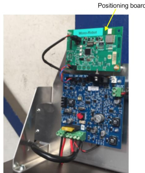
Figure 67: Location of the positioning board in the charging station
