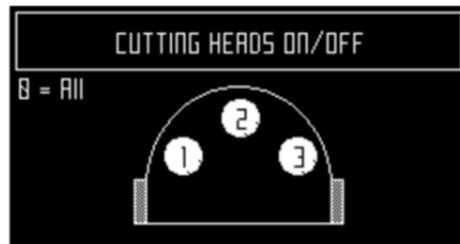
This figure indicates that all the cutting heads are enabled.
