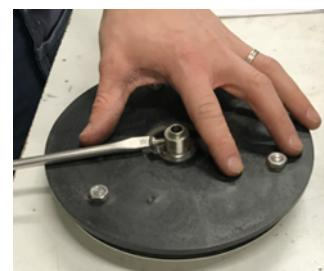
12. Place the disc assembly back onto the cutting head axle. Make sure that the screw shown above touches the flat surface of the cutting head axle as shown below.
