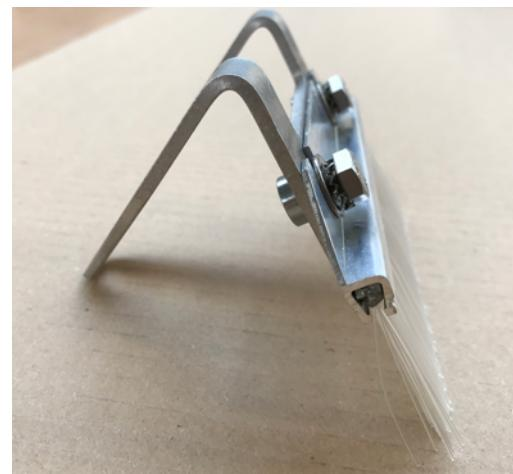
4. Screw the brushes onto the bracket, inserting the flat washer next to the brush and the crinkled washer below the screw head. Use a torque of 12Nm.
