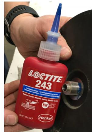
10. Replace the hexagonal washer. Tighten it to 20Nm.
