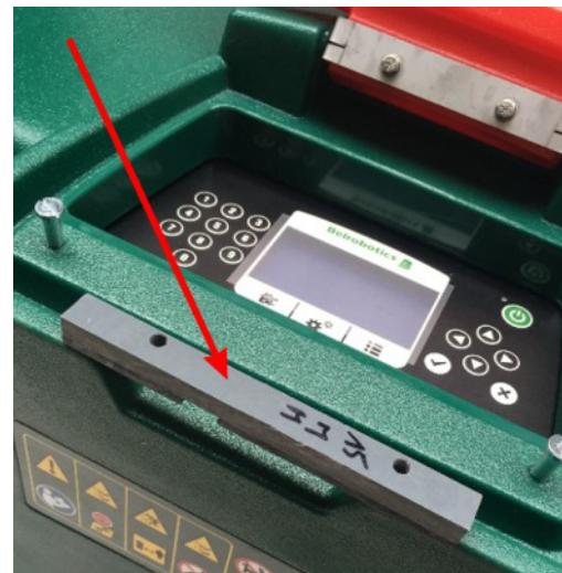
3. When the 2mm gauge is in place, close the lid and press down gently to ensure that the lid is touching the gauge.
