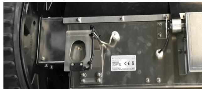
Figure 6: Identification label on the chassis
