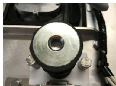
3. Fix the new silentbloc in place using the bolt underneath. Use a torque of 6Nm.
