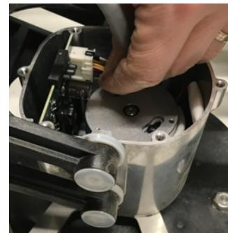
6. Visually inspect the interior of the motor. Check for dampness and dry it out if necessary.
