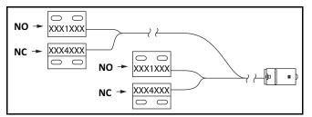
The relays are supplied as an assembly. The assembly contains two pairs of relays and the cabling between them.
