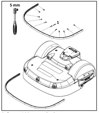
$1-B\\ umper retaining screw and washers$
