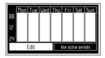
This menu shows the current schedule. The white blocks represent the time when the robot will be operating in one parcel. By default, all the times will appear white, meaning the robot will work continuously.
