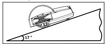
If a sloping part of the field is well away from the peripheral wire, no specific programming of the robot is required. If the sloping part of the field is near the peripheral wire, program the robot to return to the charging station by descending the slope.
