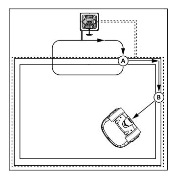
The distance traveled along the track border and the angle at which the robot turns into the field are specified in the StartZone parameters.
